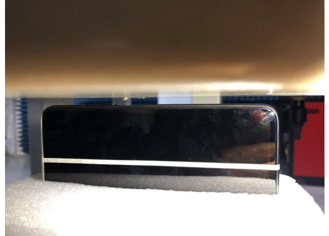
Body worn – Right (Test distance: 5mm, Thickness of DUT: 9mm)
