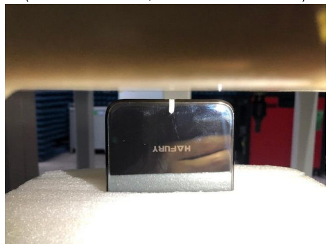
Body worn – Bottom (Test distance: 5mm, Thickness of DUT: 9mm)
