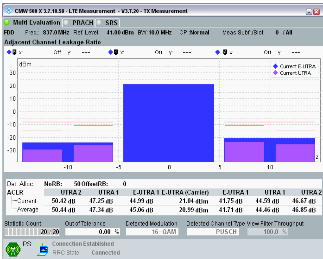
Band20 QAM16 BW=10MHz Channel=24300 RB Size=12 Position=#0.png
