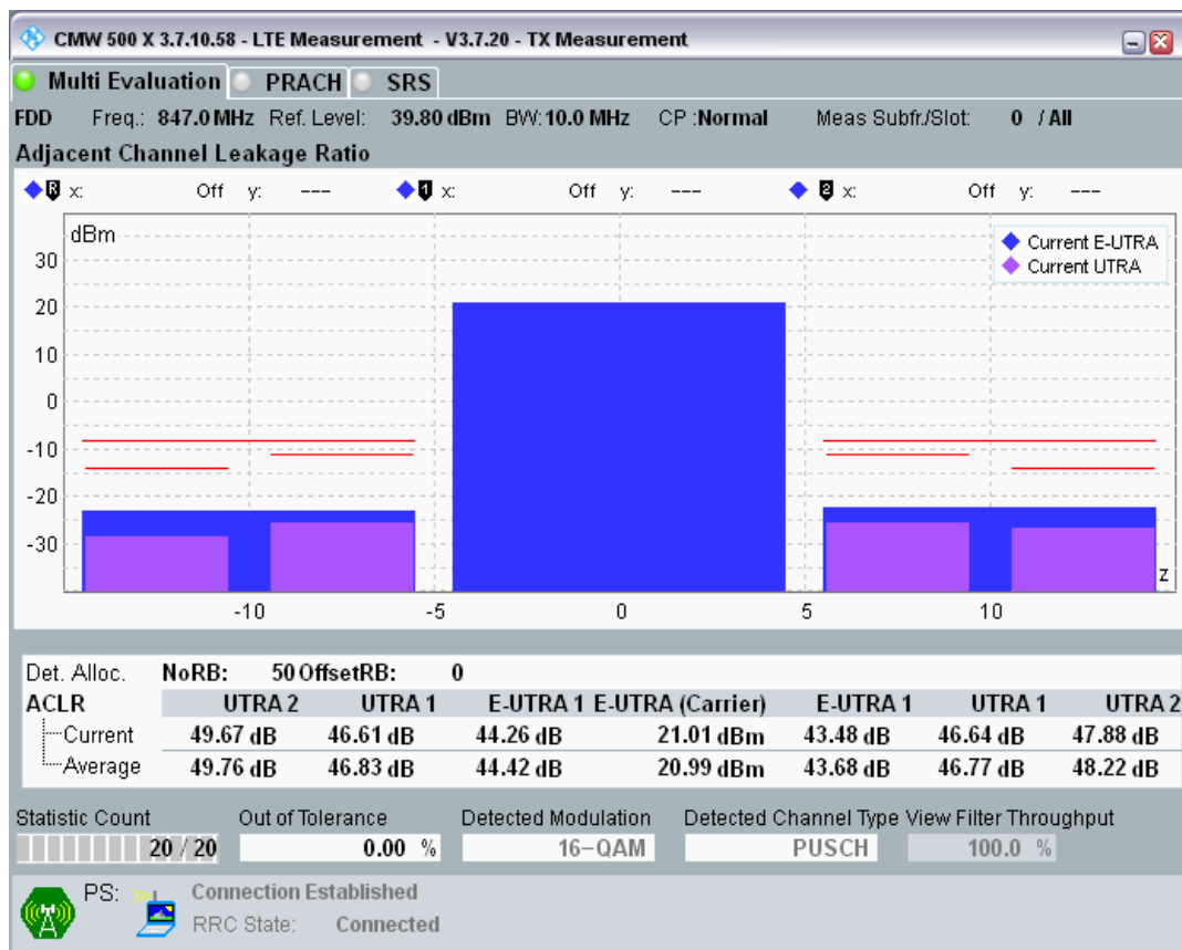
Band20 QAM16 BW=10MHz Channel=24400 RB Size=12 Position=#0.png
