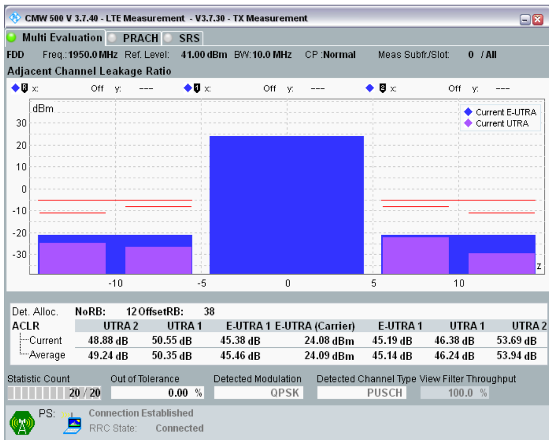
Band1 QPSK BW=10MHz Channel=18300 RB Size=50 Position=#0.png
