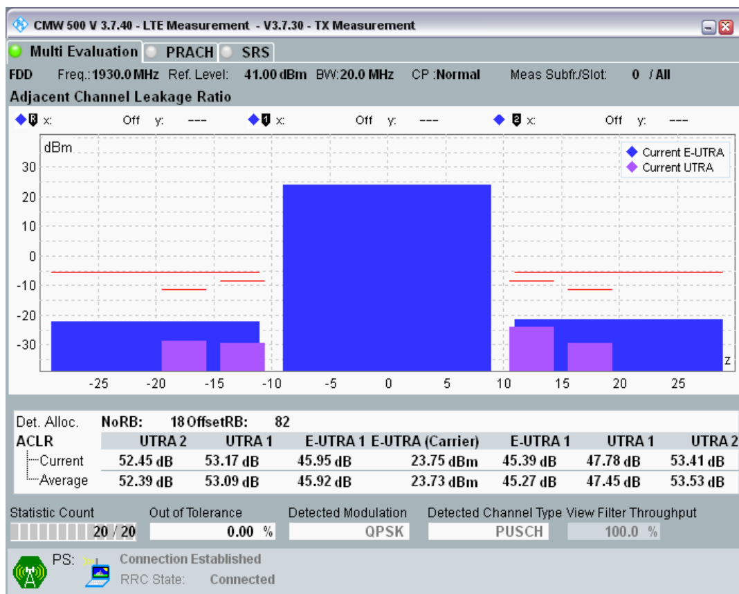
Band1 QPSK BW=20MHz Channel=18300 RB Size=100 Position=#0.png
