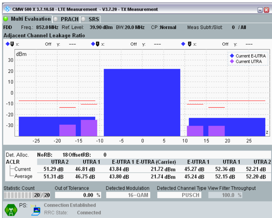
Band20 QAM16 BW=20MHz Channel=24350 RB Size=18 Position=#Max.png
