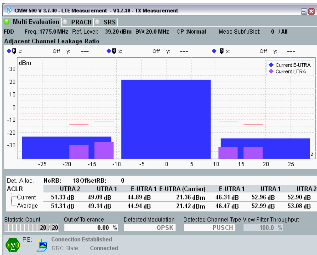
Band3 QPSK BW=20MHz Channel=19850 RB Size=18 Position=#Max.png
