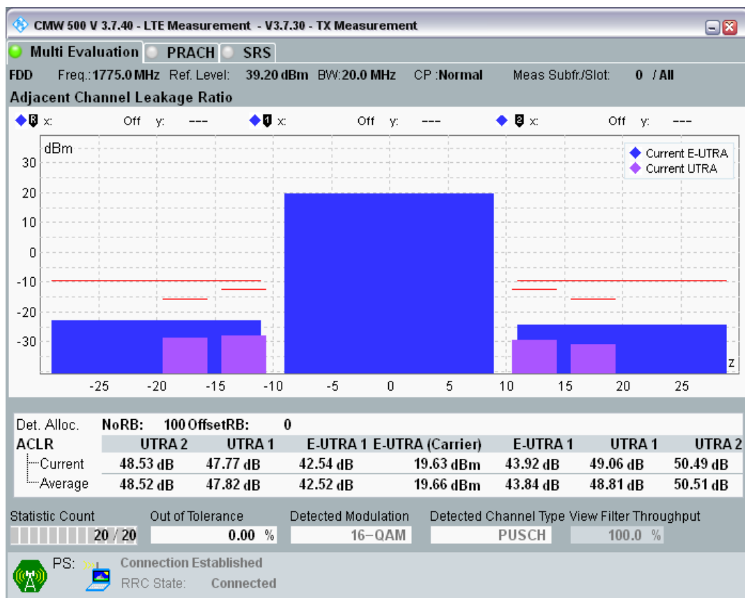
Band3 QAM16 BW=20MHz Channel=19850 RB Size=18 Position=#0.png
