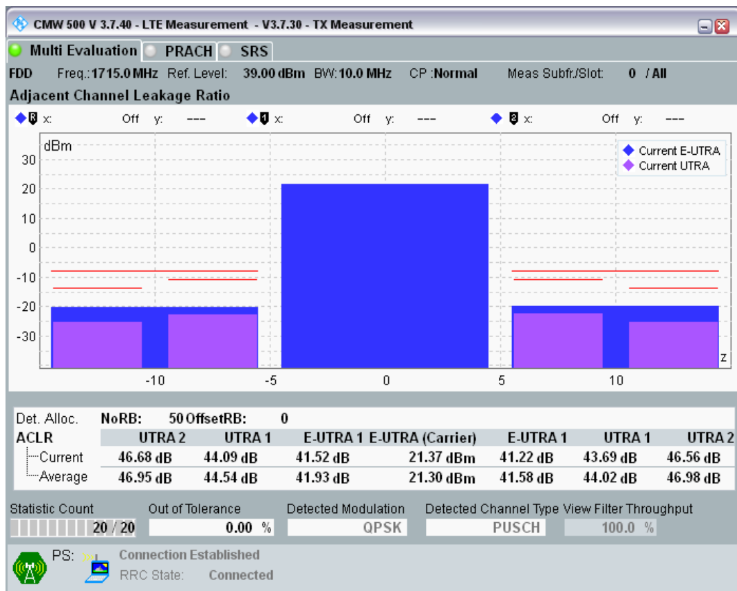
Band3 QPSK BW=10MHz Channel=19575 RB Size=12 Position=#0.png
