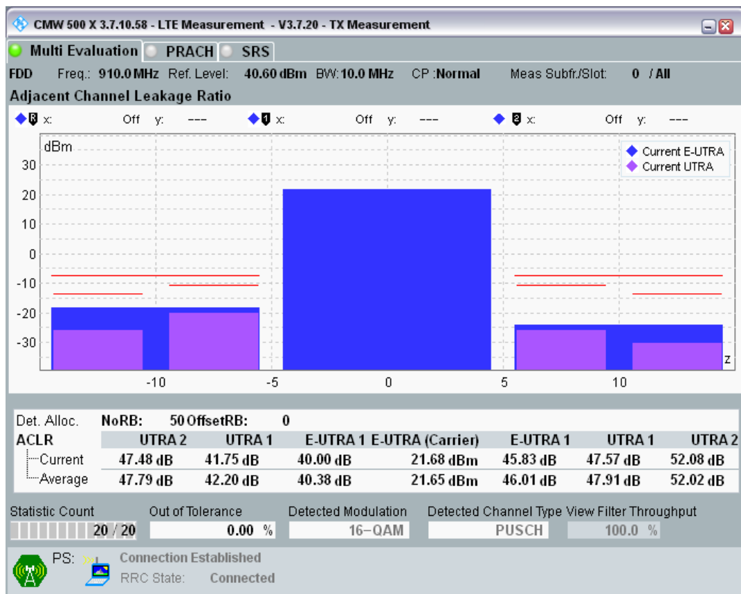
Band8 QAM16 BW=5MHz Channel=21475 RB Size=25 Position=#0.png
