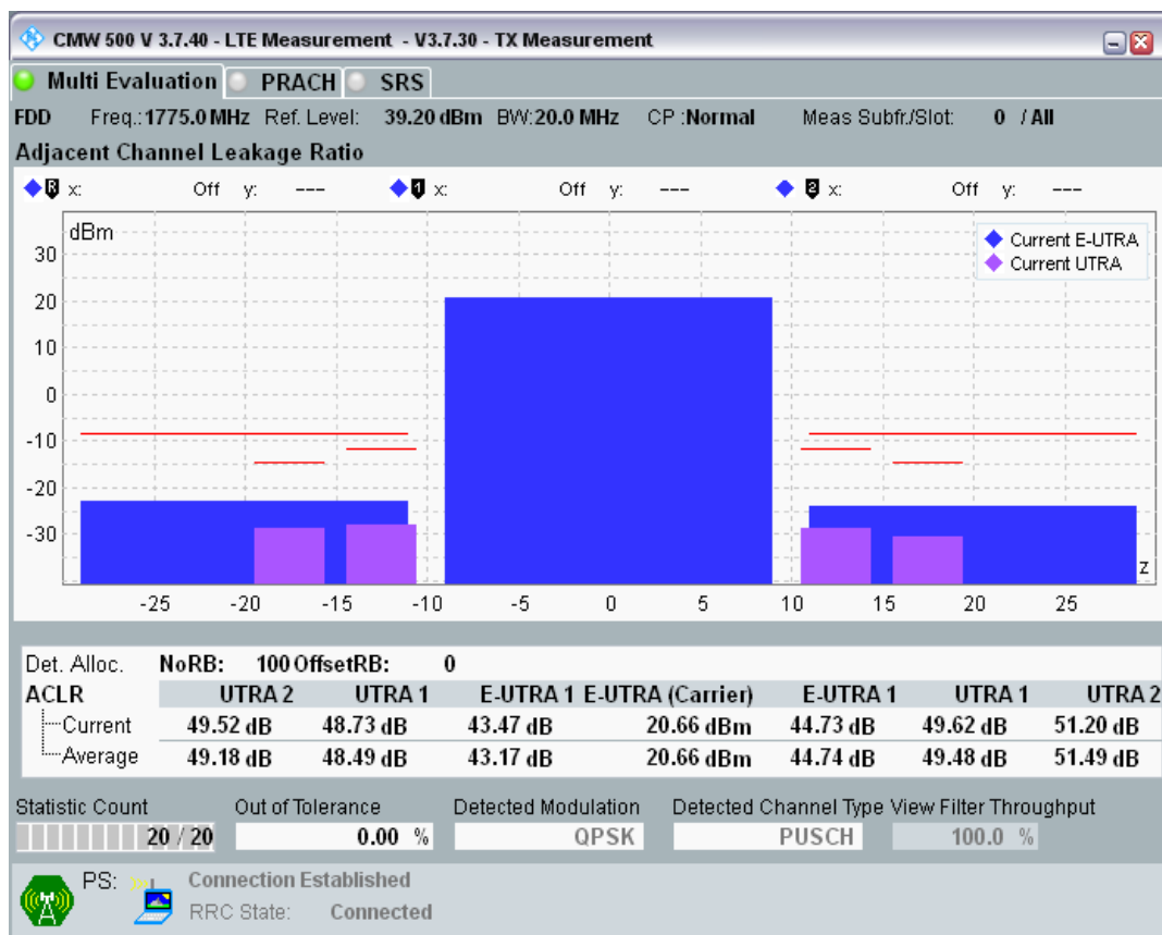
Band3 QPSK BW=20MHz Channel=19850 RB Size=18 Position=#0.png
