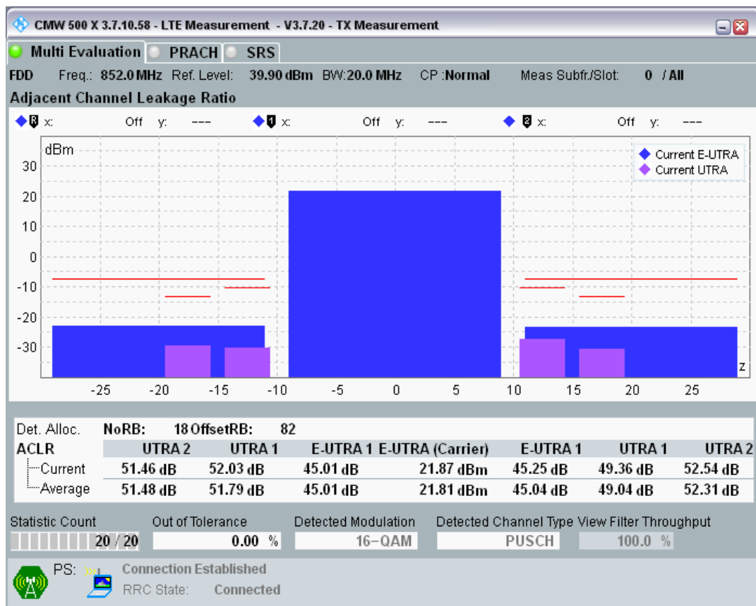
Band20 QAM16 BW=5MHz Channel=24175 RB Size=25 Position=#0.png
