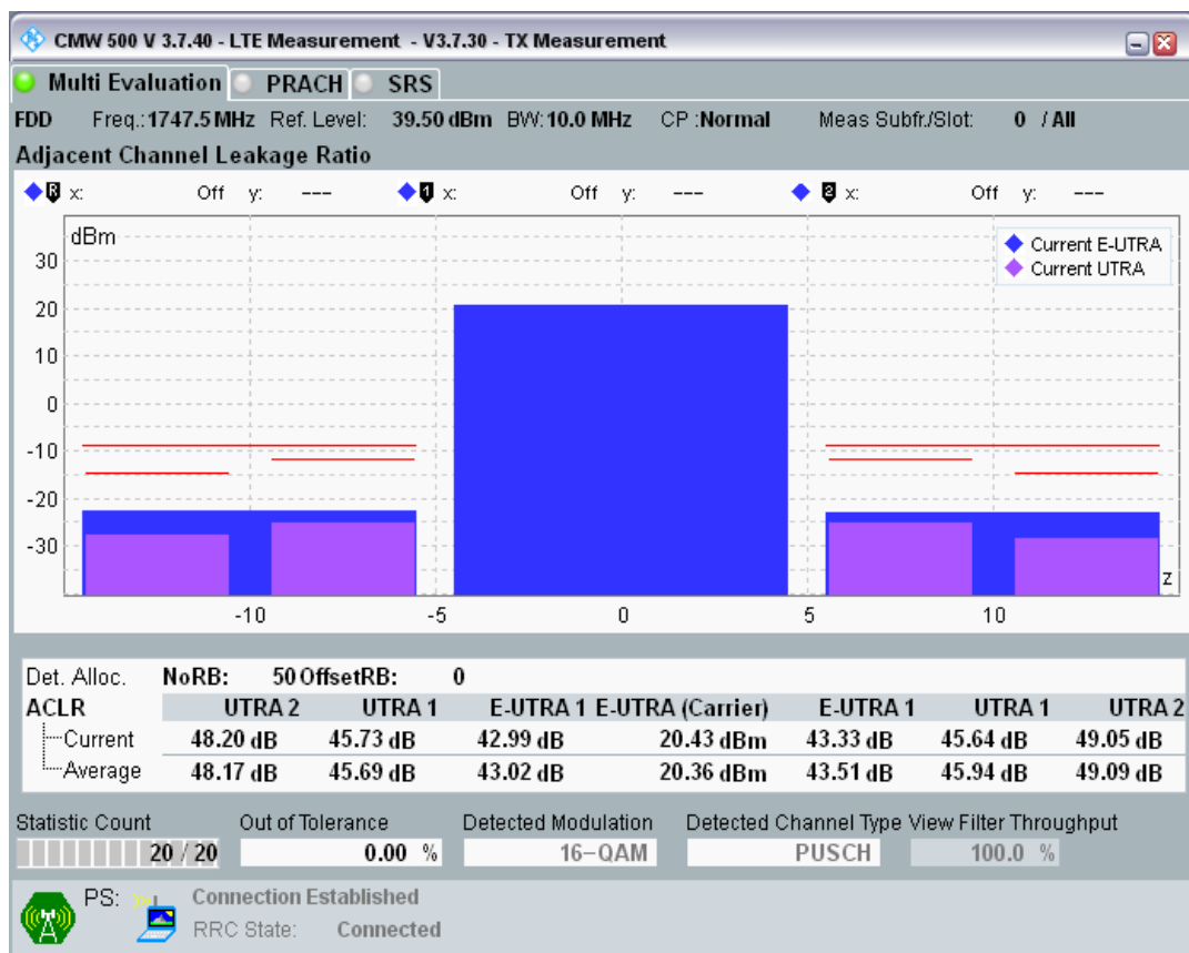
Band3 QAM16 BW=10MHz Channel=19900 RB Size=12 Position=#0.png
