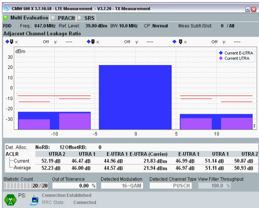
Band20 QAM16 BW=10MHz Channel=24300 RB Size=12 Position=#Max.png
