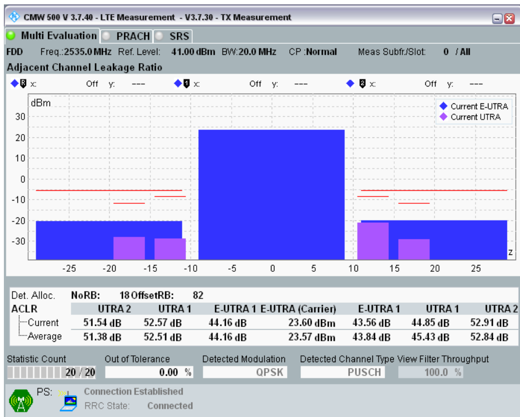
Band7 QPSK BW=20MHz Channel=21350 RB Size=100 Position=#0.png
