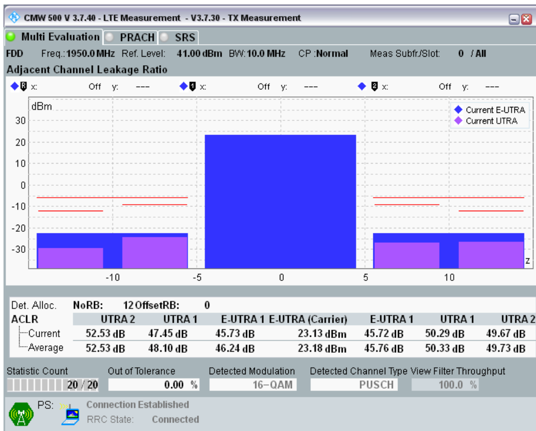
Band1 QAM16 BW=10MHz Channel=18300 RB Size=12 Position=#Max.png
