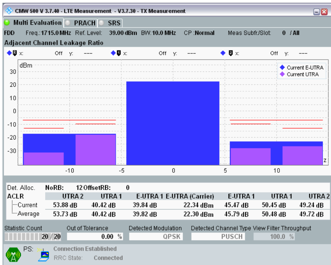
Band3 QPSK BW=10MHz Channel=19250 RB Size=12 Position=#Max.png
