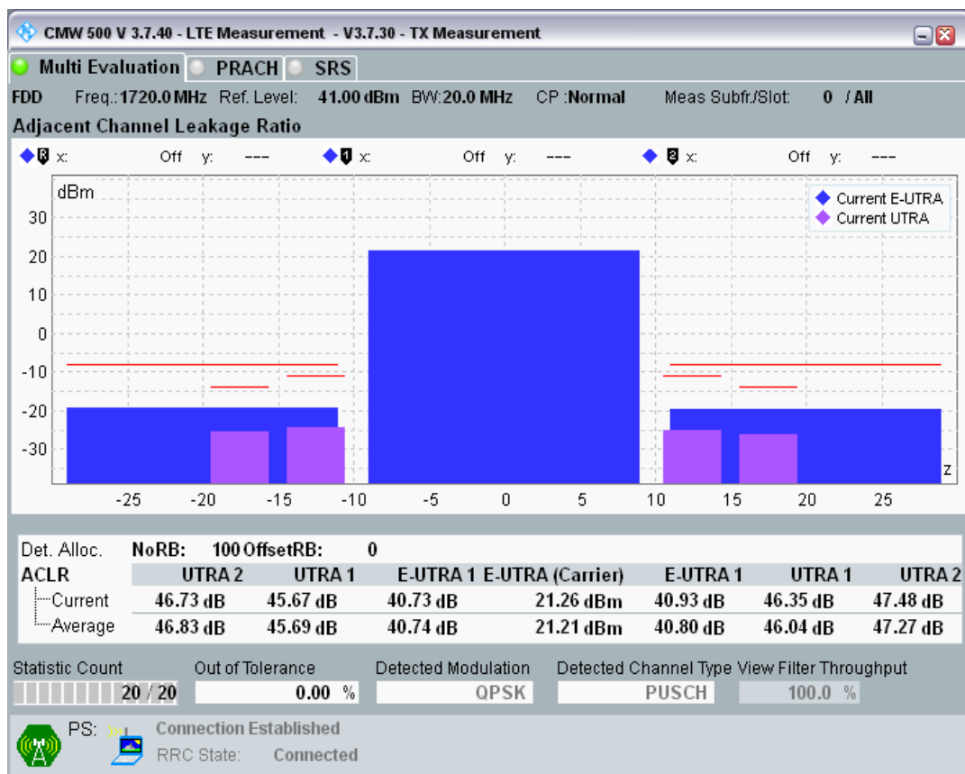
Band3 QPSK BW=20MHz Channel=19300 RB Size=18 Position=#0.png
