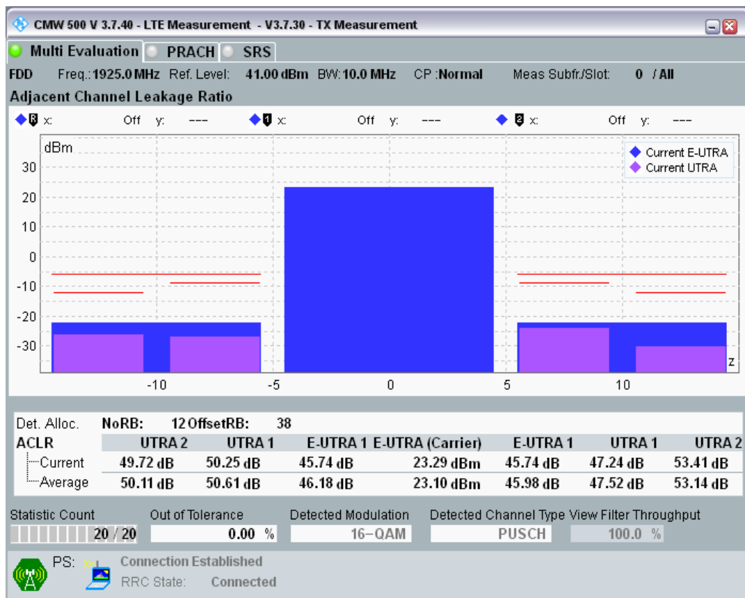
Band1 QAM16 BW=10MHz Channel=18050 RB Size=50 Position=#0.png
