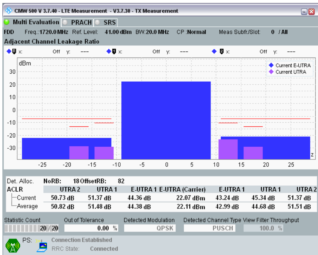
Band3 QPSK BW=20MHz Channel=19575 RB Size=100 Position=#0.png
