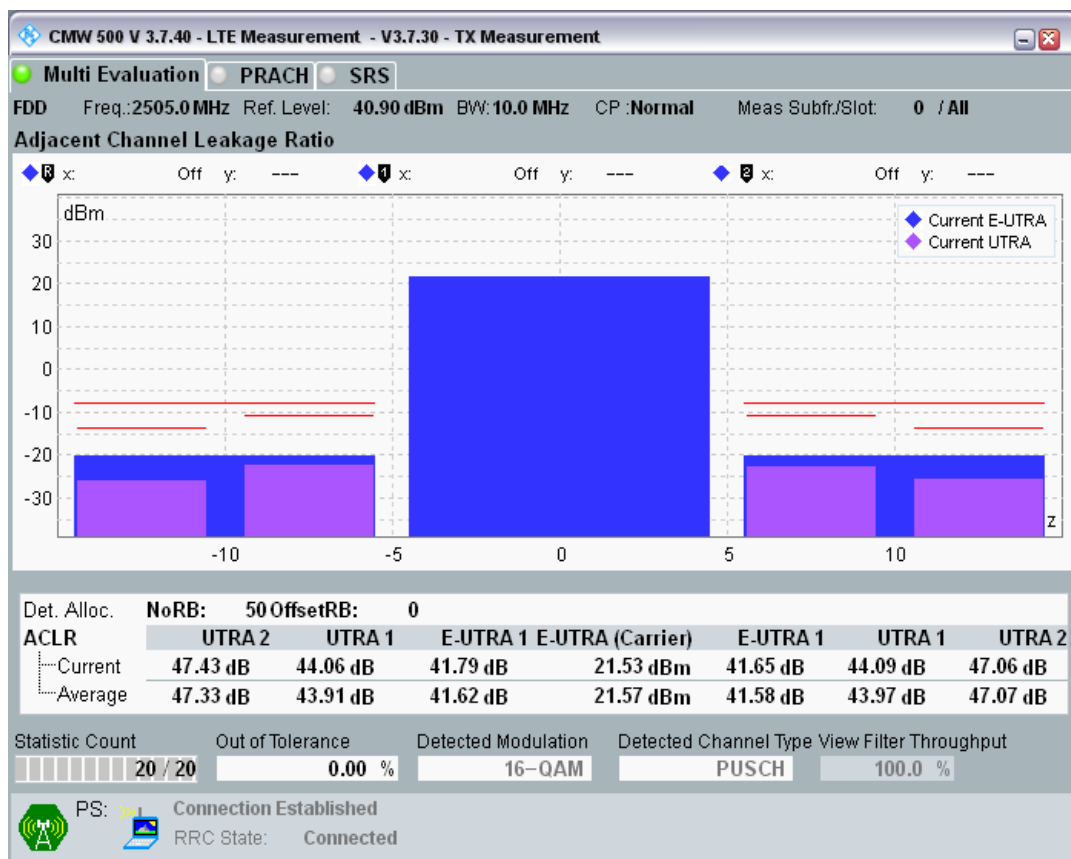
Band7 QAM16 BW=10MHz Channel=21100 RB Size=12 Position=#0.png
