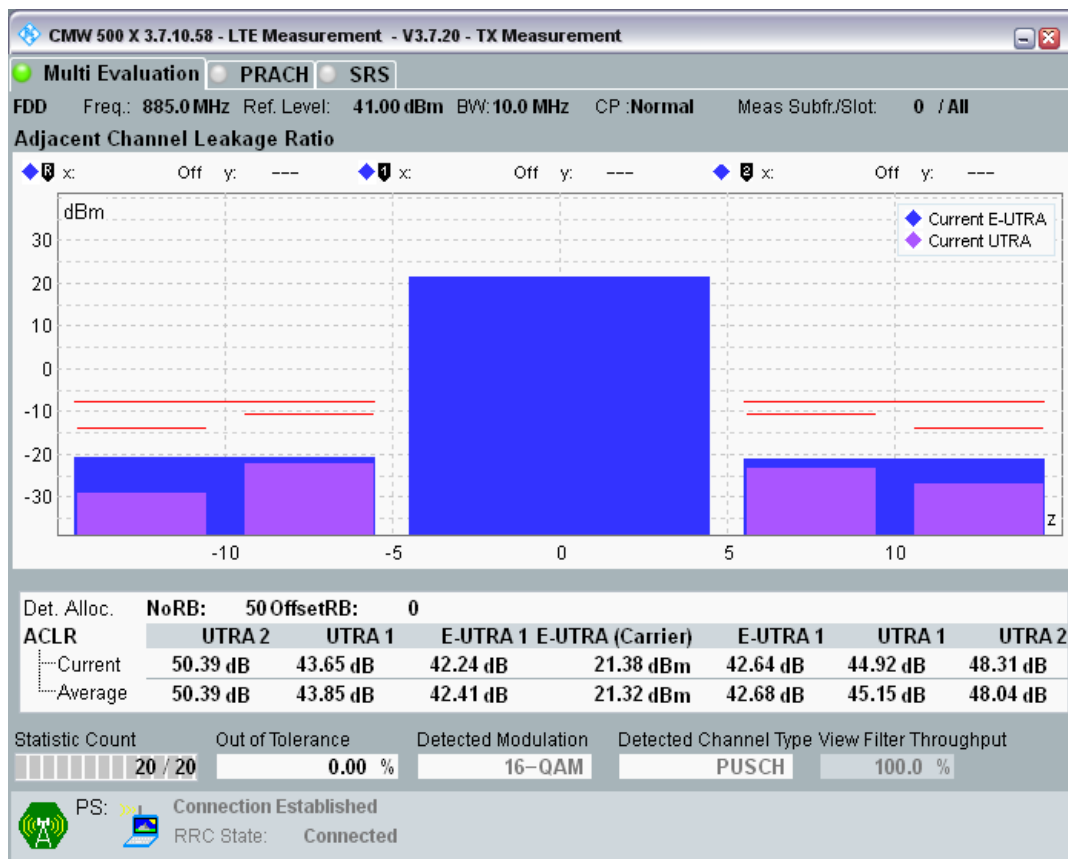
Band8 QAM16 BW=10MHz Channel=21625 RB Size=12 Position=#0.png
