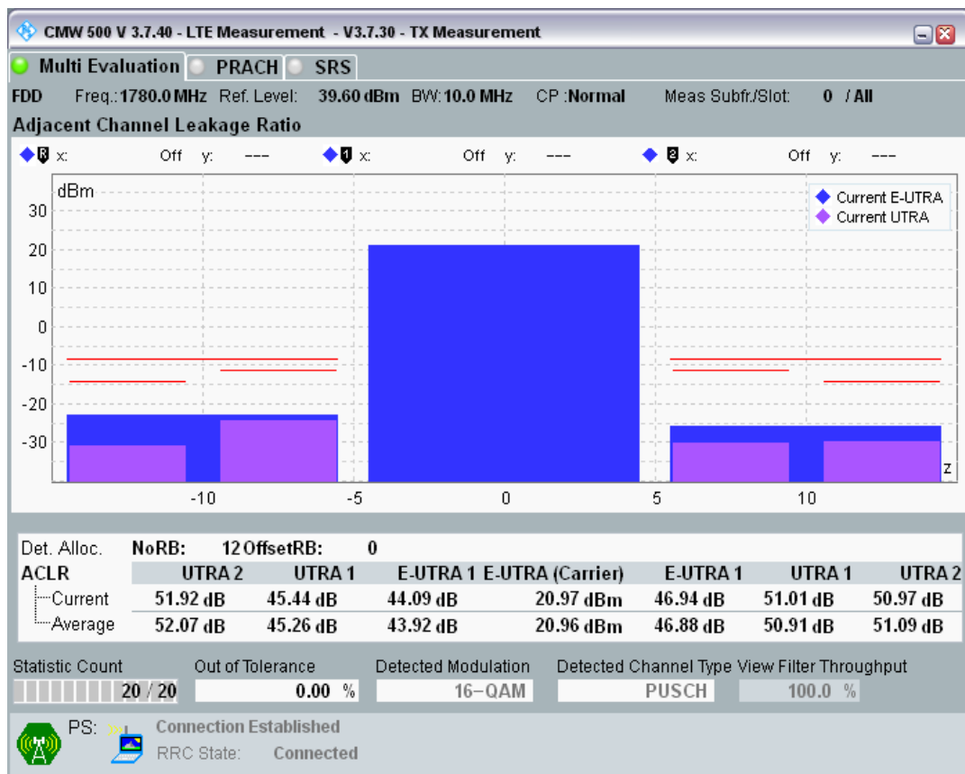
Band3 QAM16 BW=10MHz Channel=19900 RB Size=12 Position=#Max.png
