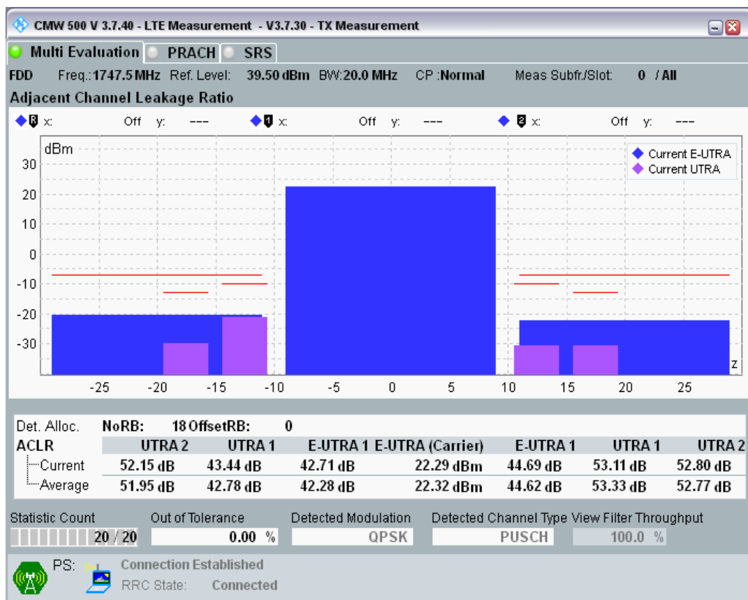
Band3 QPSK BW=20MHz Channel=19575 RB Size=18 Position=#Max.png
