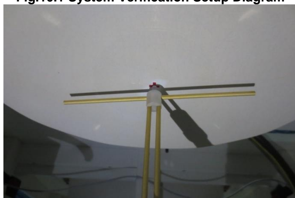
Fig.10.2 Photo of Dipole setup
