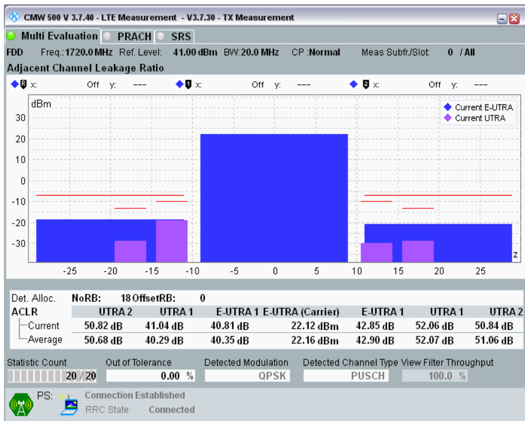
Band3 QPSK BW=20MHz Channel=19300 RB Size=18 Position=#Max.png
