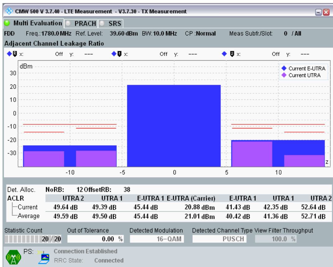
Band3 QAM16 BW=10MHz Channel=19900 RB Size=50 Position=#0.png
