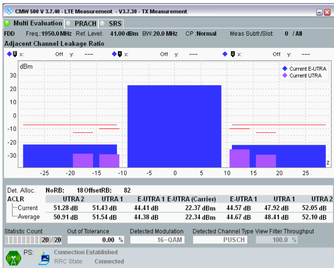
Band1 QAM16 BW=20MHz Channel=18500 RB Size=100 Position=#0.png
