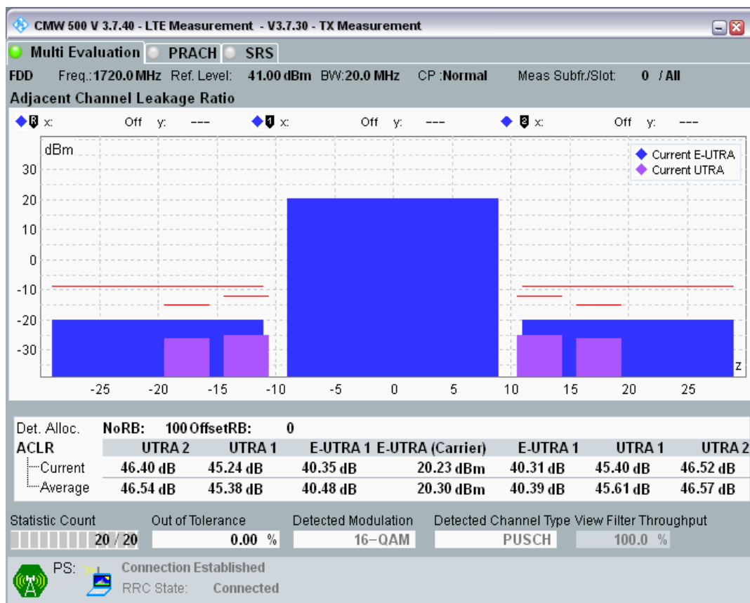
Band3 QAM16 BW=20MHz Channel=19300 RB Size=18 Position=#0.png
