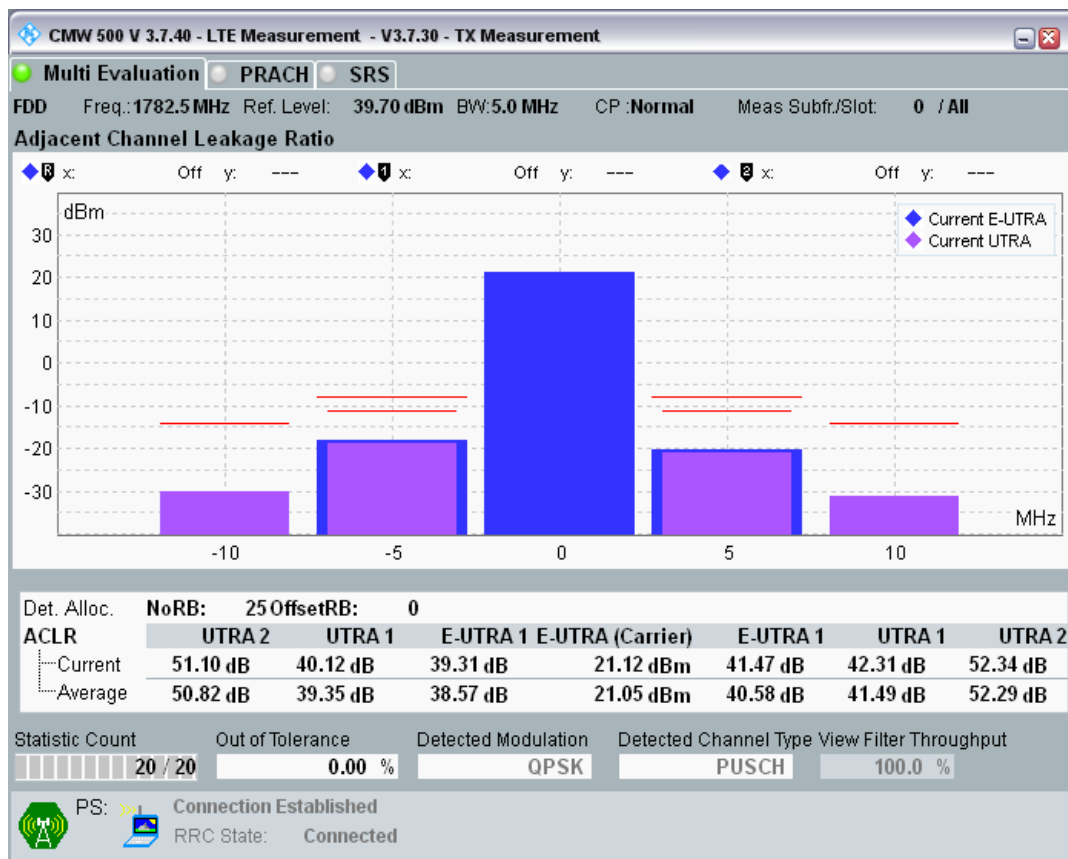
Band3 QPSK BW=5MHz Channel=19925 RB Size=8 Position=#0.png
