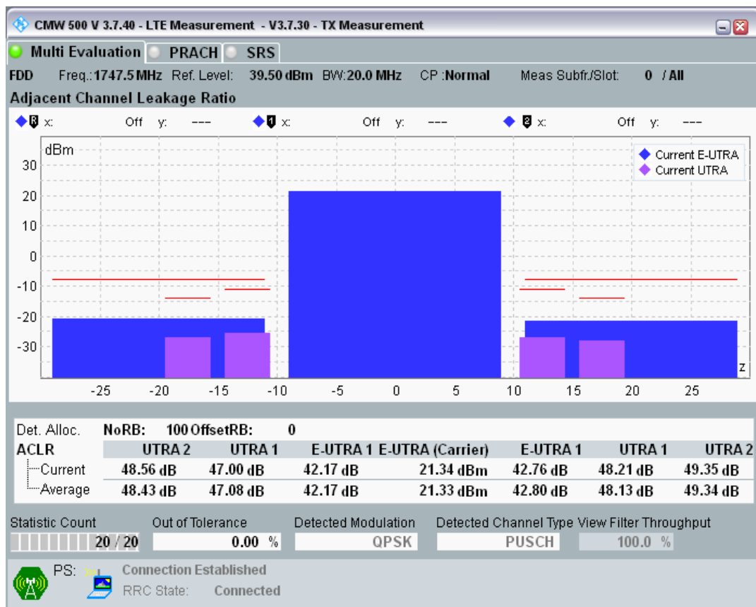
Band3 QPSK BW=20MHz Channel=19575 RB Size=18 Position=#0.png
