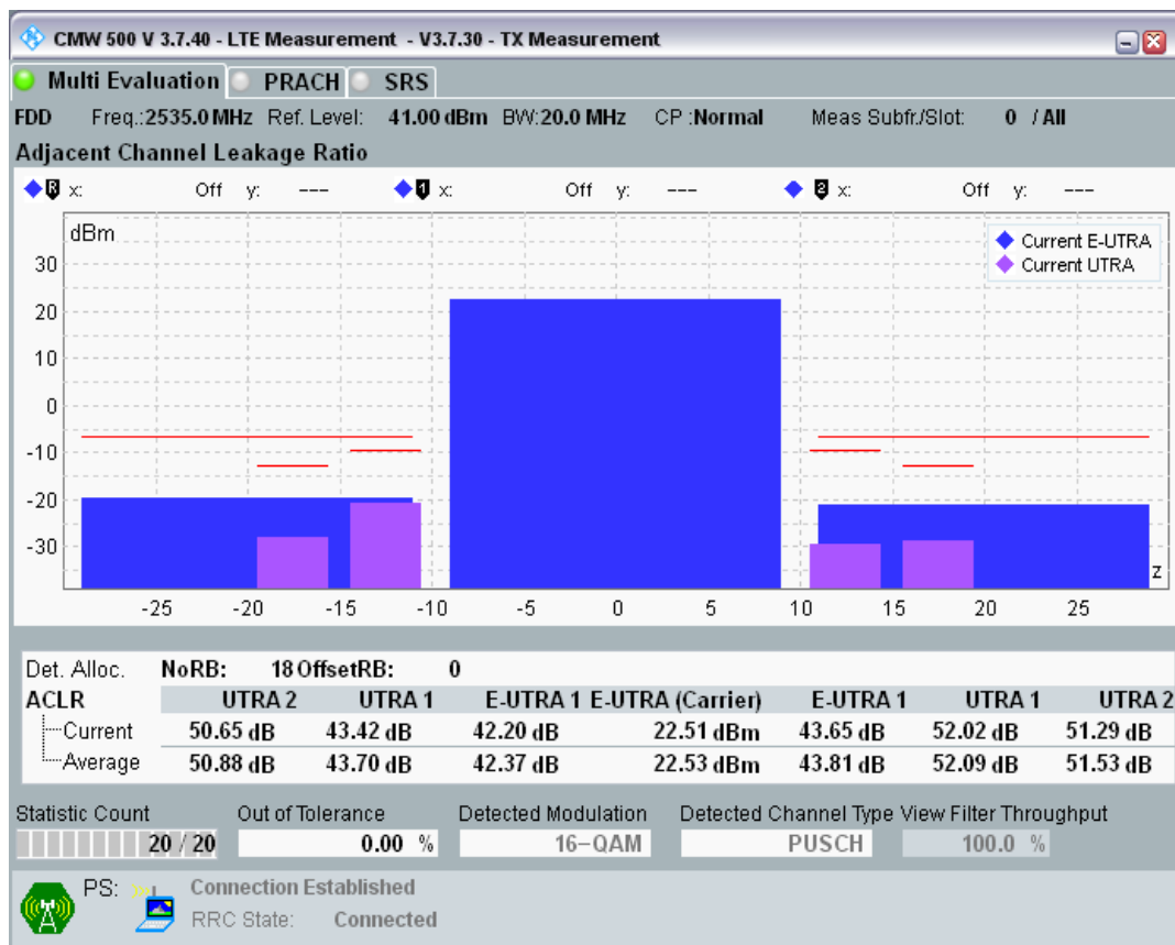
Band7 QAM16 BW=20MHz Channel=21100 RB Size=18 Position=#Max.png
