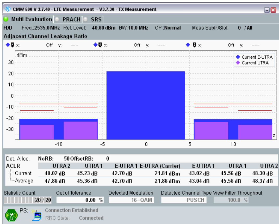
Band7 QAM16 BW=10MHz Channel=21400 RB Size=12 Position=#0.png
