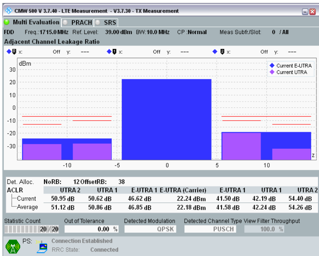
Band3 QPSK BW=10MHz Channel=19250 RB Size=50 Position=#0.png
