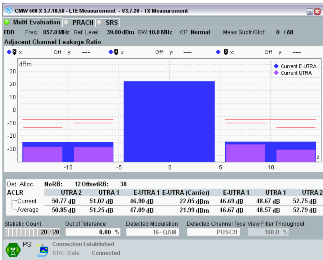
Band20 QAM16 BW=10MHz Channel=24400 RB Size=50 Position=#0.png
