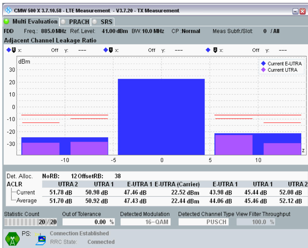
Band8 QAM16 BW=10MHz Channel=21500 RB Size=50 Position=#0.png
