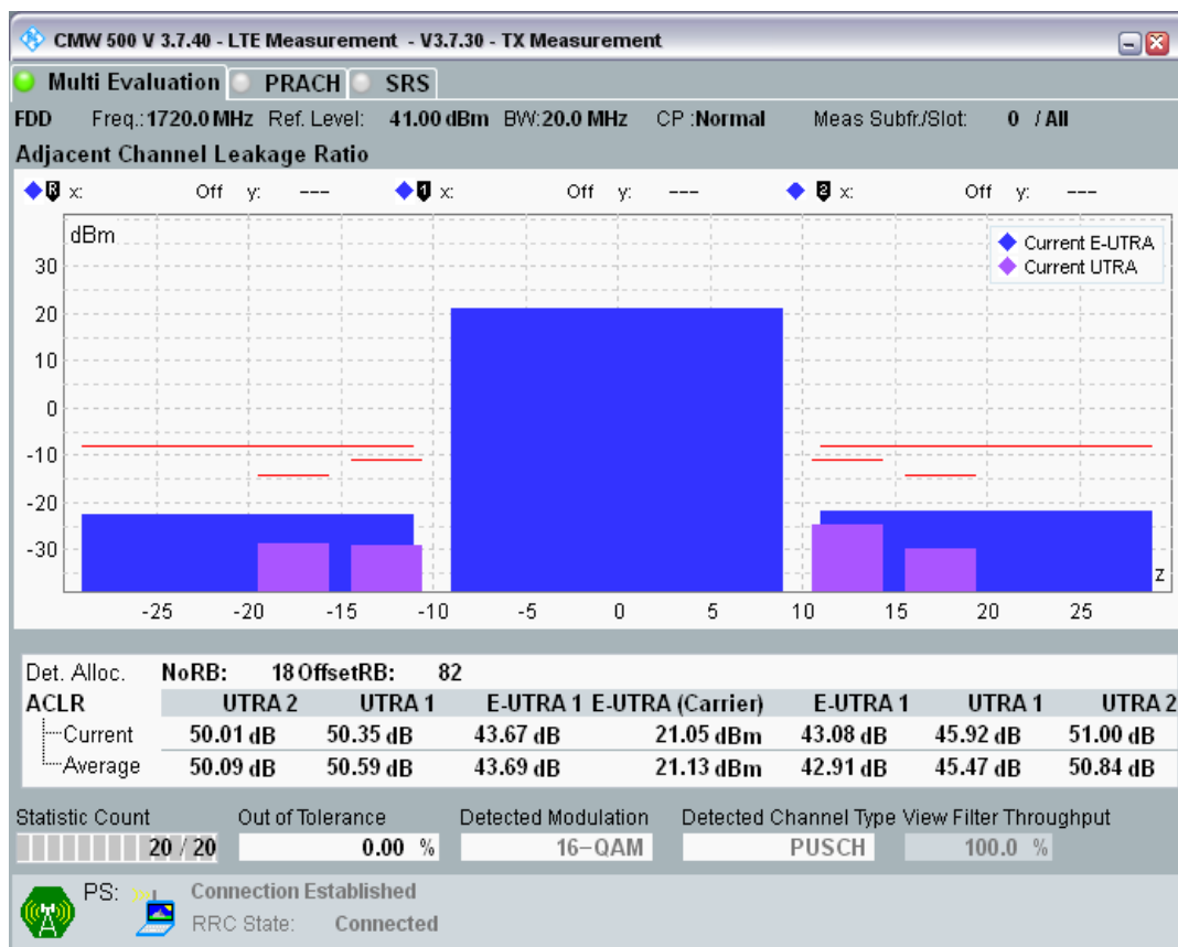
Band3 QAM16 BW=20MHz Channel=19575 RB Size=100 Position=#0.png
