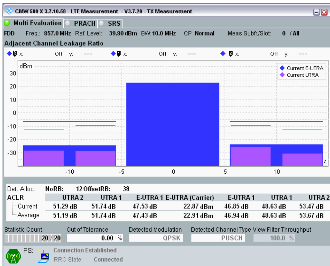
Band20 QPSK BW=10MHz Channel=24400 RB Size=50 Position=#0.png
