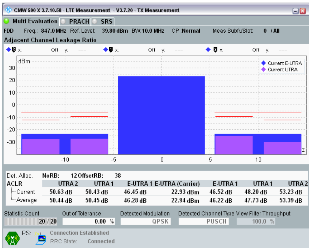
Band20 QPSK BW=10MHz Channel=24300 RB Size=50 Position=#0.png
