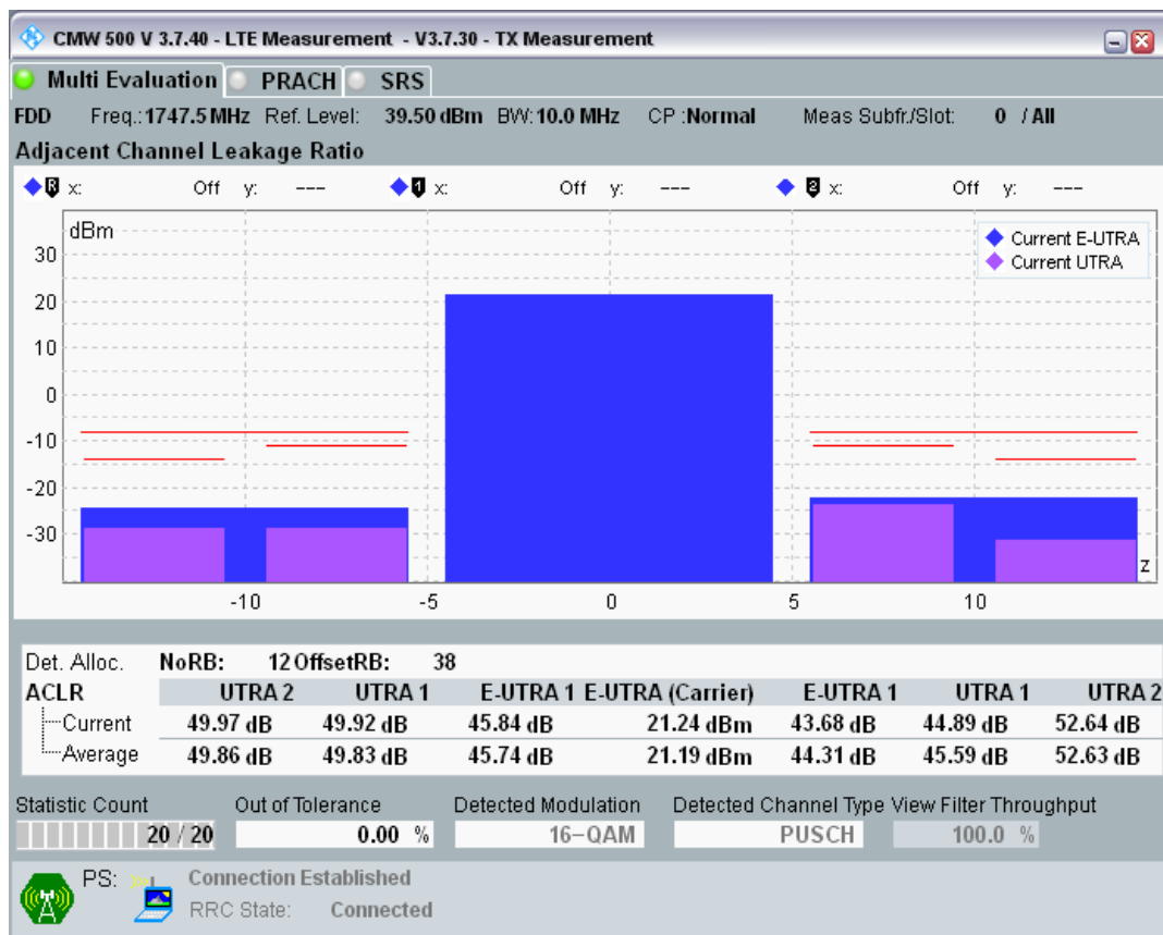
Band3 QAM16 BW=10MHz Channel=19575 RB Size=50 Position=#0.png
