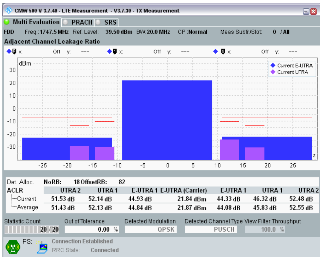
Band3 QPSK BW=20MHz Channel=19850 RB Size=100 Position=#0.png
