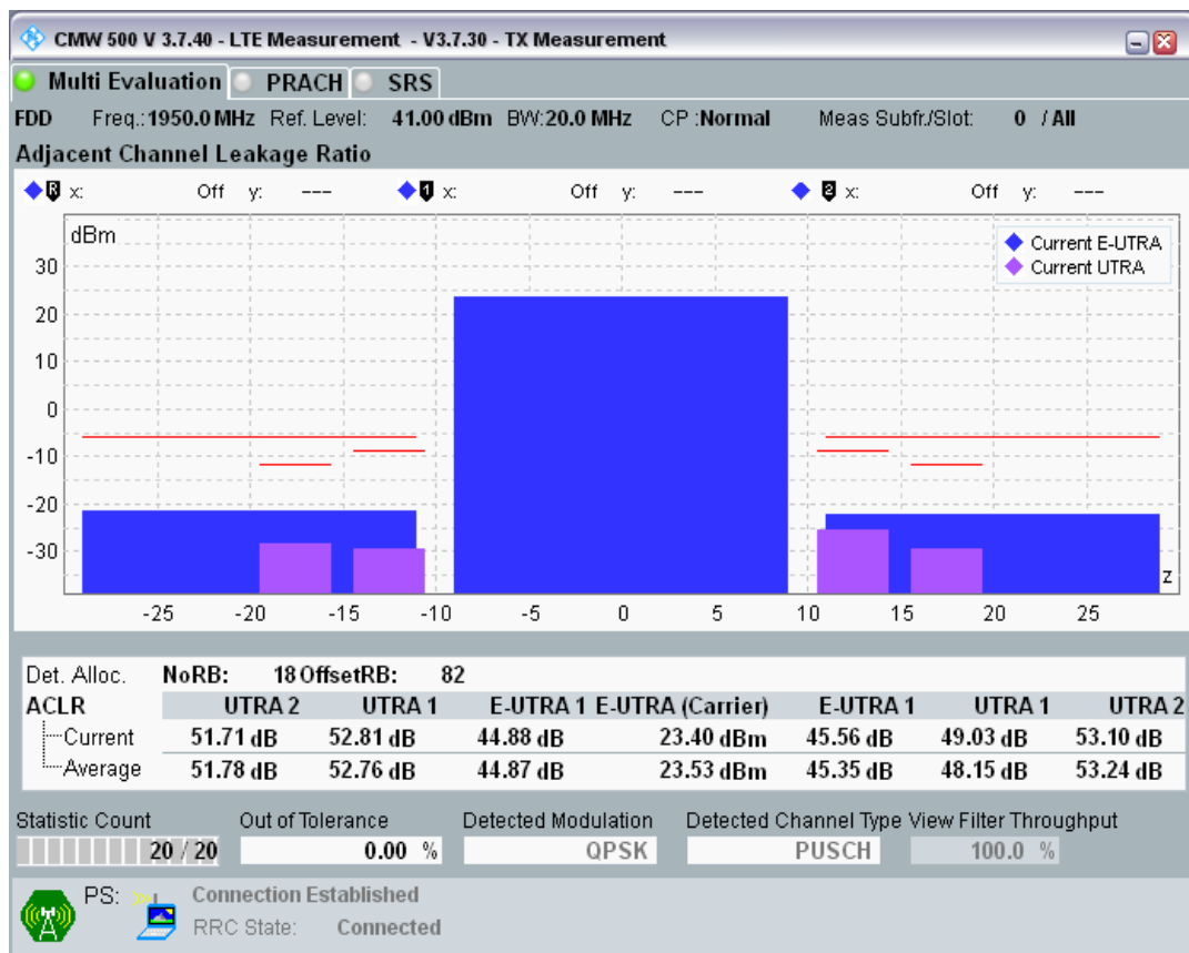
Band1 QPSK BW=20MHz Channel=18500 RB Size=100 Position=#0.png
