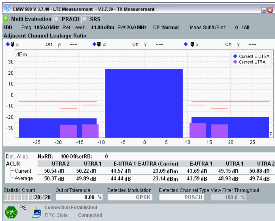
Band1 QPSK BW=20MHz Channel=18300 RB Size=18 Position=#0.png
