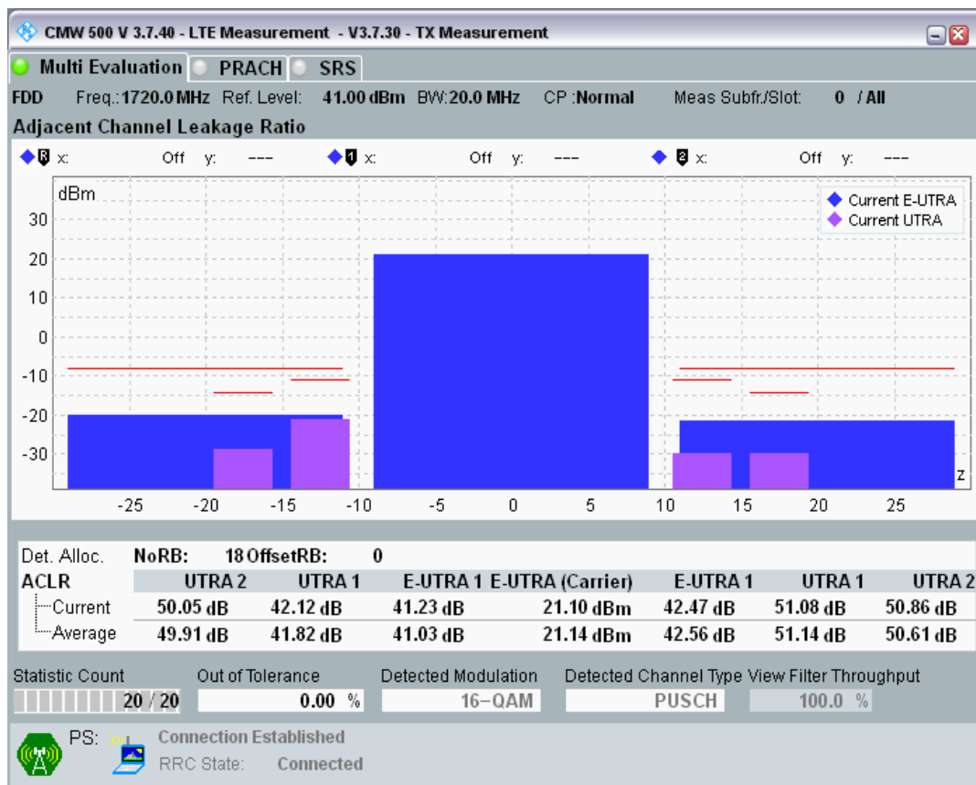
Band3 QAM16 BW=20MHz Channel=19300 RB Size=18 Position=#Max.png
