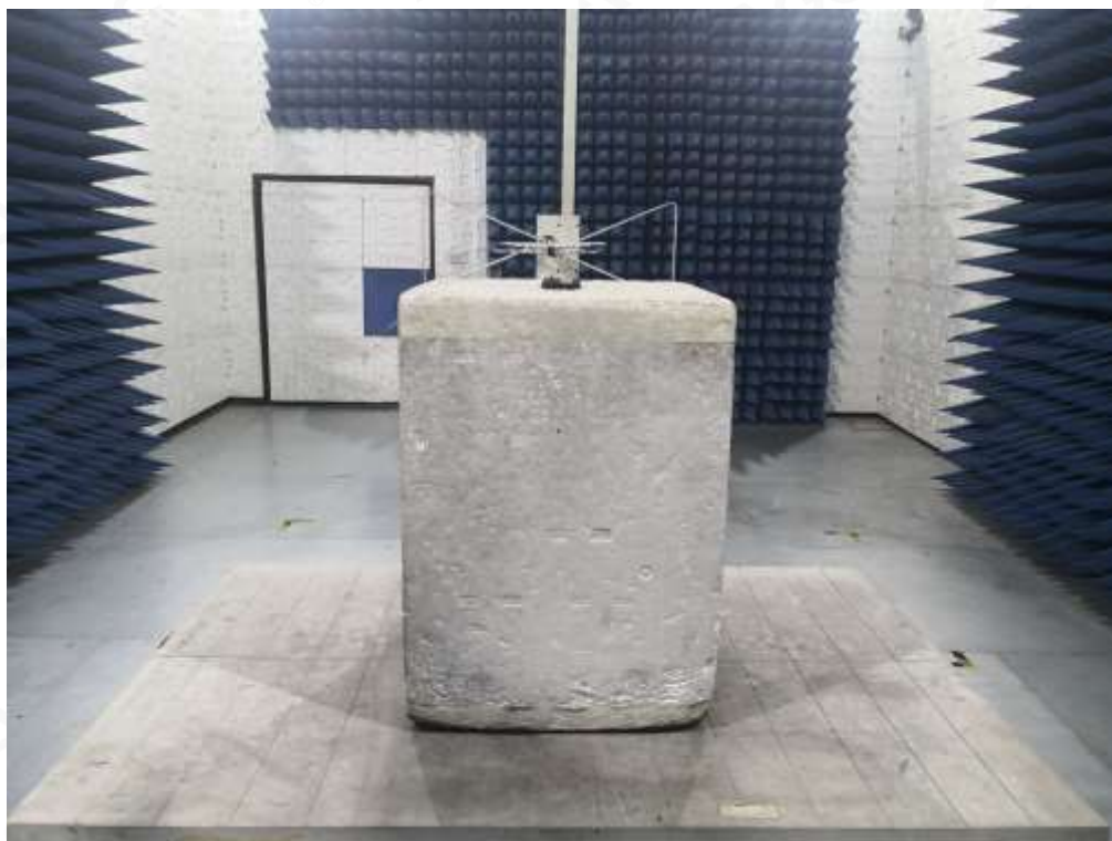
RADIATED SPURIOUS EMISSION ABOVE 1G TEST SETUP
