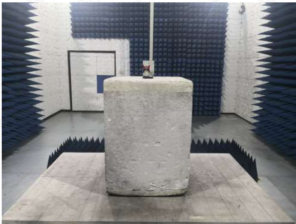
RADIATED SPURIOUS EMISSION ABOVE 1G TEST SETUP
