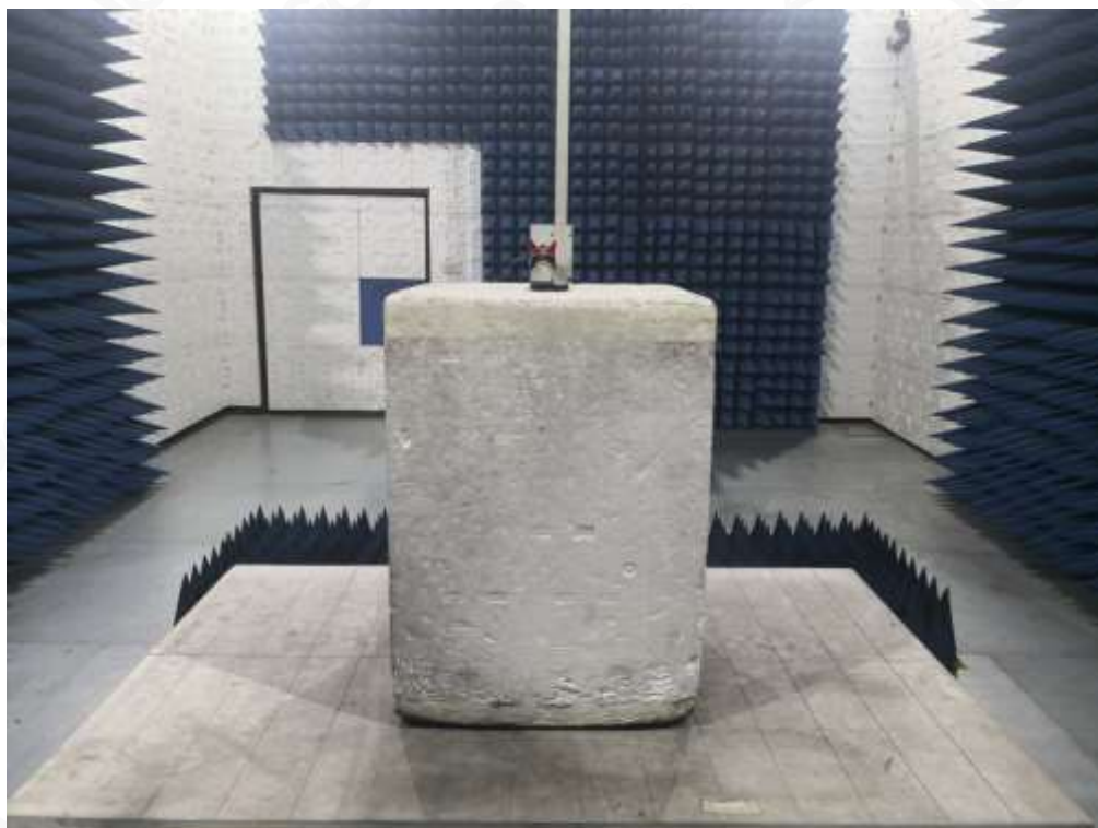
RADIATED SPURIOUS EMISSION ABOVE 1G TEST SETUP
