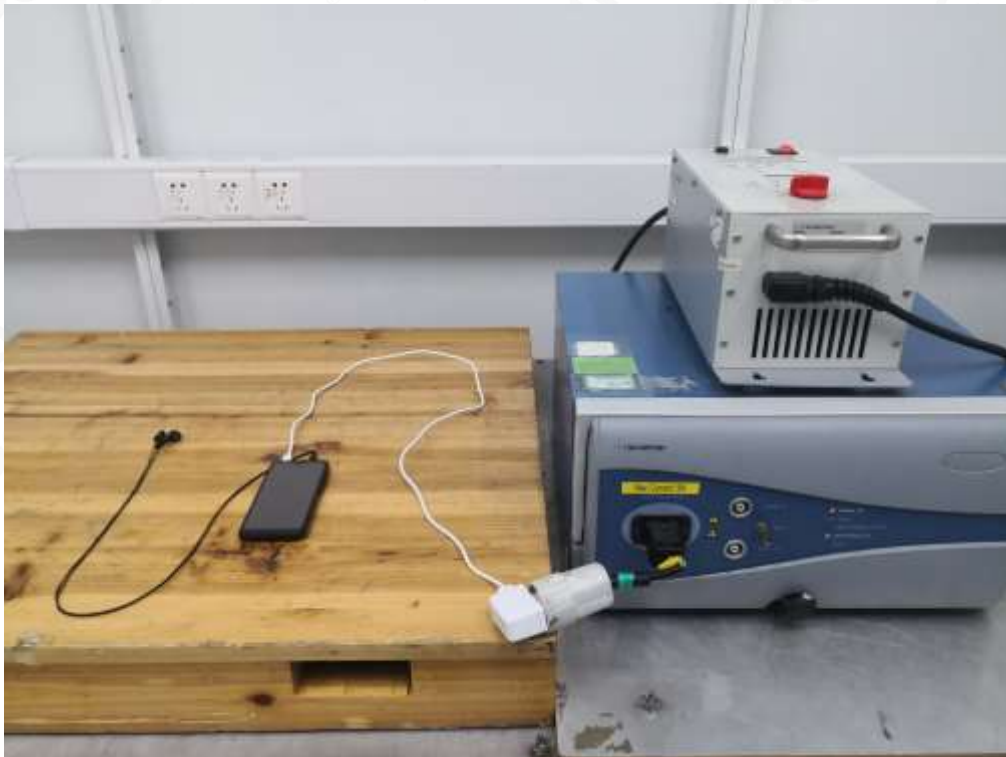
EFT SURGE and DIPS IMMUNITY TEST SETUP
