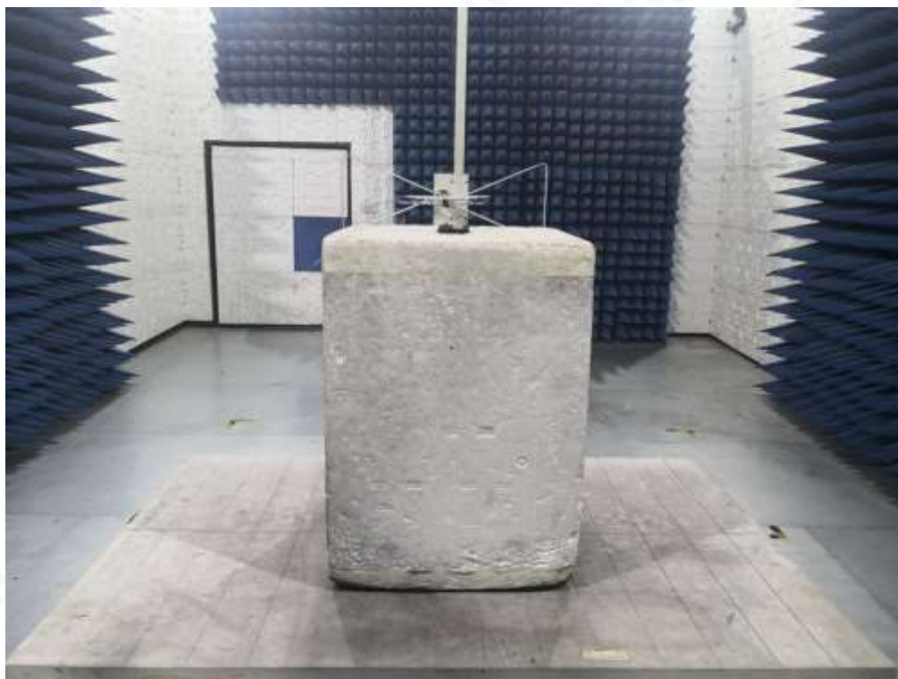
RADIATED SPURIOUS EMISSION ABOVE 1G TEST SETUP
