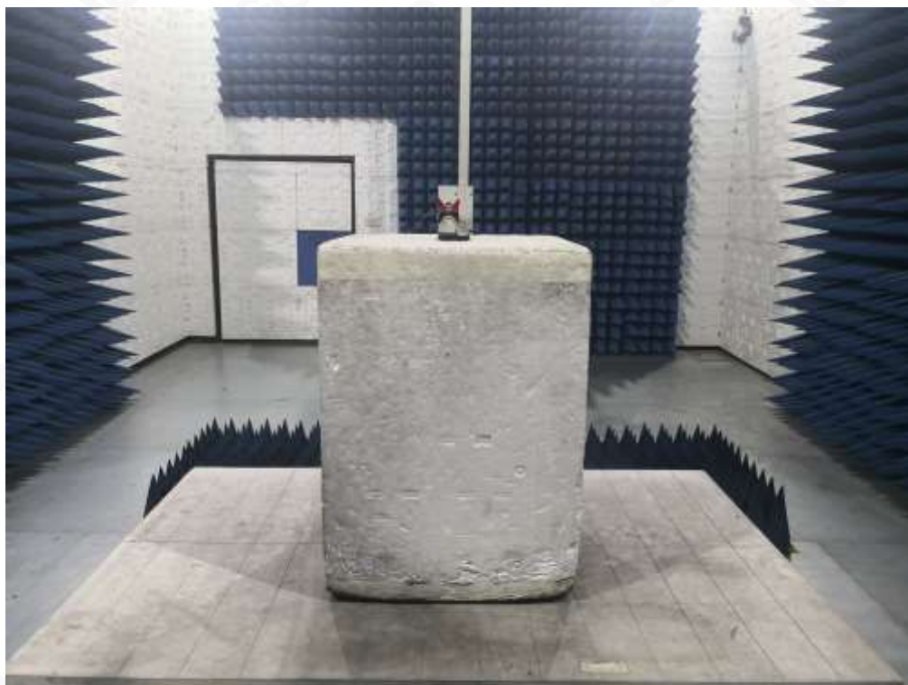
RADIATED SPURIOUS EMISSION ABOVE 1G TEST SETUP
